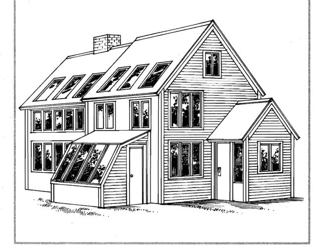
Consider the contribution of solar energy (indicated by insolation values for your region) and natural processes (including breezes and shade) to the heating and cooling of the home, in order to avoid oversizing a backup heating system or air conditioner. A home that is oriented to true south, is tightly constructed and well insulated, and has operable windows for air circulation should not require large fossil-fuel burning equipment to maintain thermal comfort.
