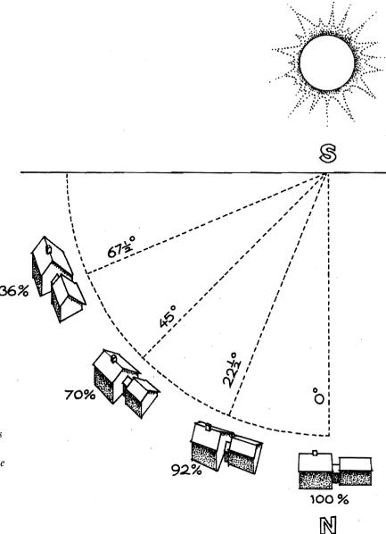
The ideal orientation for a solar house is with its long axis perpendicular to true south (or 0° on the diagram). Because of various factors, it's sometimes necessary to shift the orientation somewhat. Within 20 degrees of true south, the cost in solar gain is minimal, but as the orientation shifts more drastically, the house will significantly lose solar benefits.
